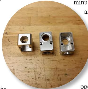
With the new Brother Speedio machine, the customer was able to use the same tooling, but crank up the spindle speed and feed rates and achieve a cycle time of under 8 minutes, all while achieving better and more consistent surface finishes on the critical deep pocket milling operations.
