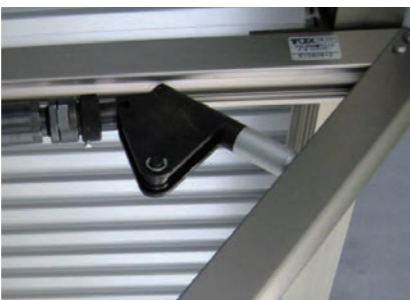
45 Angle nose of AR2000A-45 offers smooth riveting at hard-to-reach place
