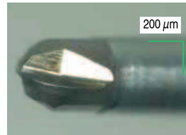
Tool damage after milling 10 hours.
